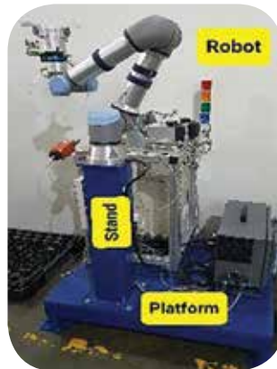
Examples of manufacturing aids used for injection moulding and automation processes such as robot platforms, arm attachments and assembly aids.
