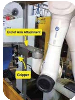
Examples of manufacturing aids used for injection moulding and automation processes such as robot platforms, arm attachments and assembly aids.
