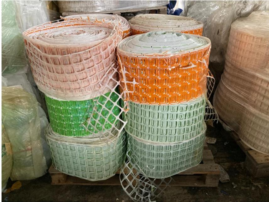
*Picture 2: PS Skirt Trim left over from the manufacture of packaging items such as food containers, lids and blister packs can be recycled into materials for the production of thicker sheets to make sturdier nonfood packaging related parts such as vehicle door inside panels, sports equipment and dunnage trays used in transport.*
